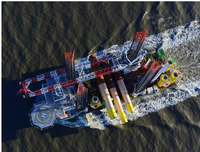
GeoSea's Innovation installation vessel carries N1 foundation pieces out to sea; installation of the project's first monopile was successfully completed on December 14<sup>th</sup>.
